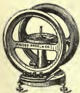
FIG. 3.—Helmholtz Tangent Galvanometer.
